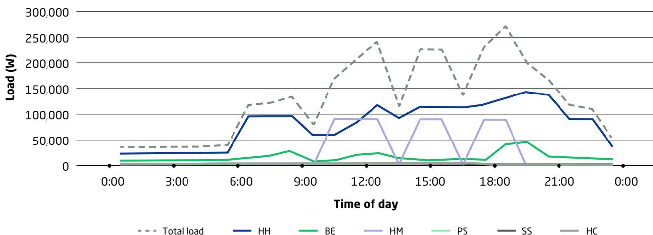
Given the anticipated load profile, the hydropower plant is estimated to have a power capacity of 272 kW, and a maximum annual energy demand of 1.15 GWh in year 19. It is assumed that the energy production matches the energy demand, which results in a load factor of 48%.
