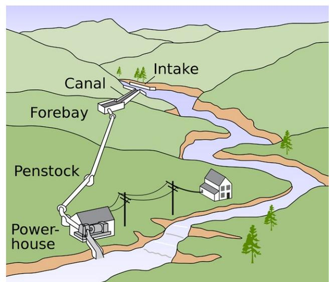
**FIGURE 3.** Typical layout for a small hydropower plant
