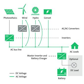
Solar PV generation by its nature undergoes cyclical intermittency within a day and seasonal variations across a year. A solar PV system for a mini-grid must be designed to generate at an optimal level and supply electricity to meet the current and forecasted demand, bearing in mind that system sizing and components have implications for both the cost and quality of electricity produced. There are four typical design options for solar PV mini-grids:
