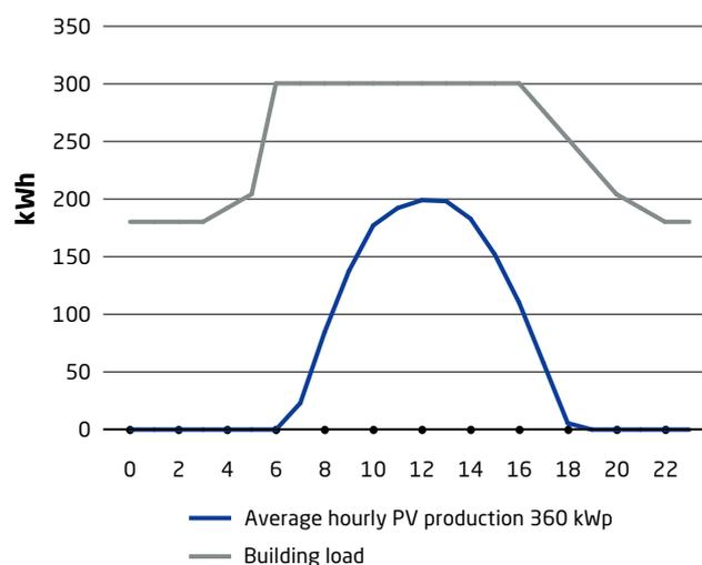
The estimated annual energy yield of the PV system is approximately 1,418 kWh/kWp using PVsyst software, after considering system losses, temperature, cloud cover and panel soiling. Power outages and poor power quality frequency ranges from 1.6%
