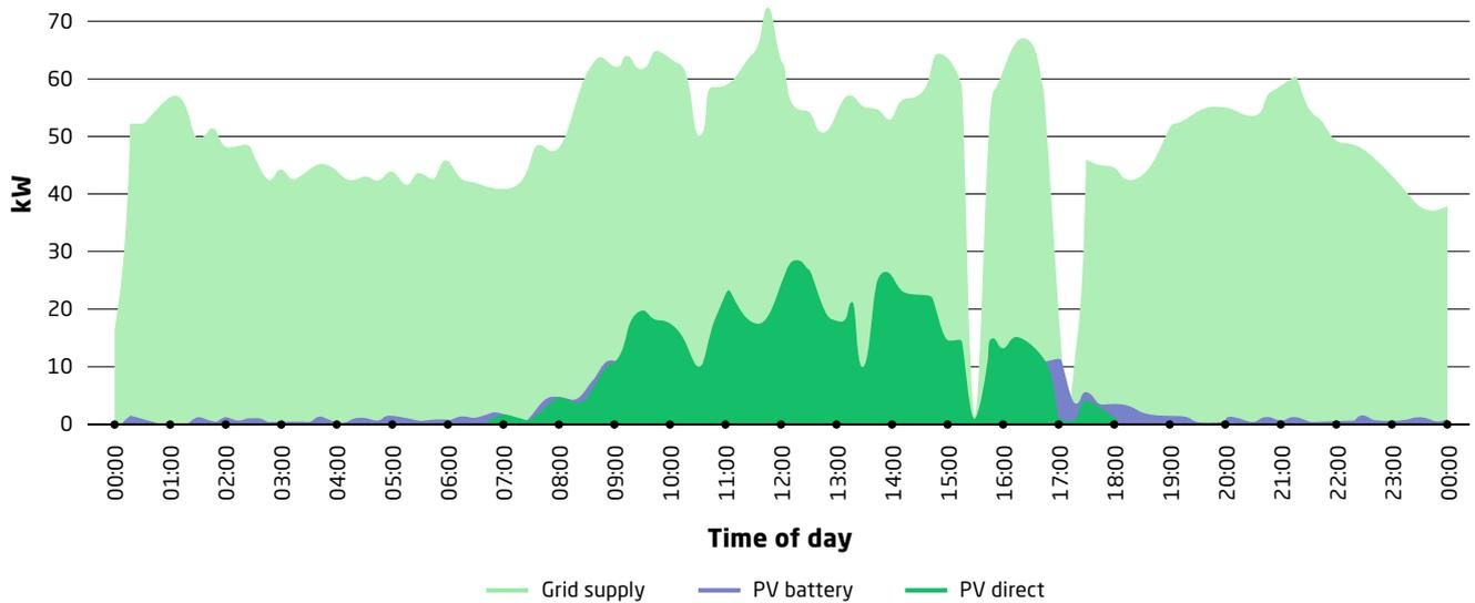
**FIGURE 12.** Example of PV system generation vs. consumption over a month in Kampala
