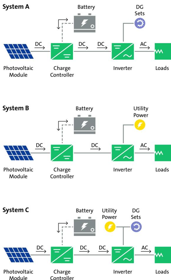
Solar PV systems can be installed on the ground or on the roof of a building (approximately 10–15 m<sup>2</sup> of space is needed per kW). For ground-mounted installation, shading is a relevant consideration while for roof-mounted systems the orientation and load bearing capacity of the roof (usually at least 20 kg/m<sup>2</sup>) are important. Fixed-tilt systems are most common.
