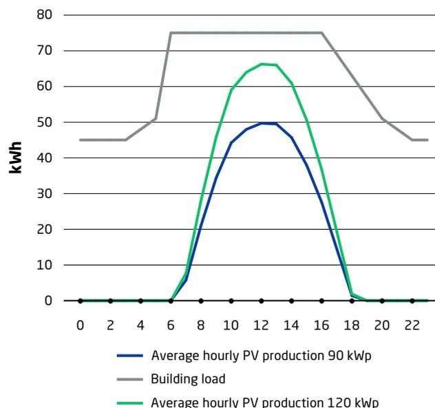
**FIGURE 2. 300 kW peak load vs. average hourly PV output**
